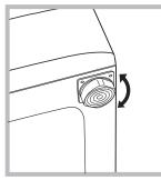
Your machine may make a considerable amount of noise if the two front feet have not been adjusted correctly. 1. Install the washing machine on a flat sturdy floor, without resting it up against walls, furniture cabinets or other. 2. If the floor is not perfectly level, compensate for any unevenness by tightening or loosening the adjustable front feet (see figure); the angle of inclination, measured according to the worktop, must not exceed 2°.
